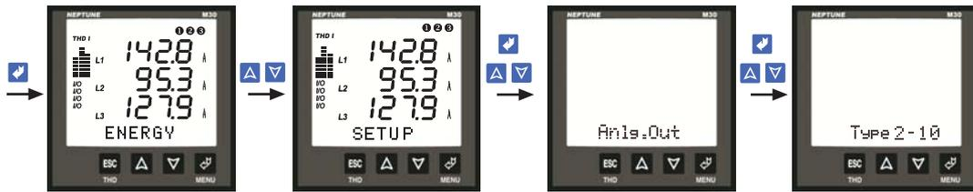
In device, this feature gives the possibility that observing the measured values by other devices with converting these values in to 0-10 V or 2-10 V voltage data. The below parameters can be set as analog output in device.
