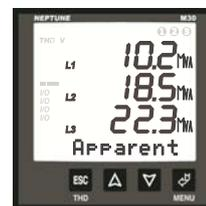
**$\Sigma$ Powers** Measured total active, total reactive and total apparent power values
