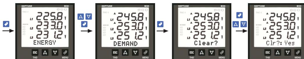
Figure 53: Clearing the max. VLN
