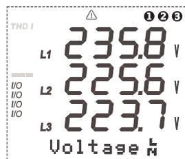
**Figure 1:** The existence of three phases on LCD.
