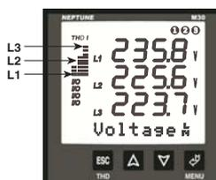
At the bottom of the screen, the active sub-menu is displayed. Each bar on the left indicates the ratio between total harmonic amount of current or voltage for each phase as a percentage value. Each step is 10%. It is possible to switch between "THD V" and "THD I" by ESC button. Also, it is possible to see the numerical values of the THD values by going to the Instantaneous Values Menu.
