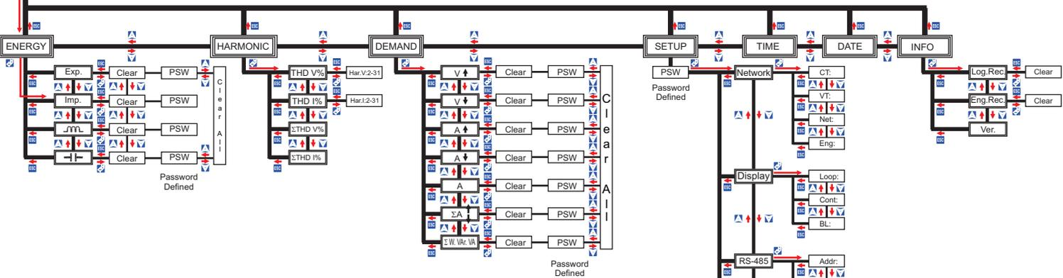
Blue symbols are the front buttons of M30 and they show how the progress, which is shown in red arrows, can be done with regarding buttons.
