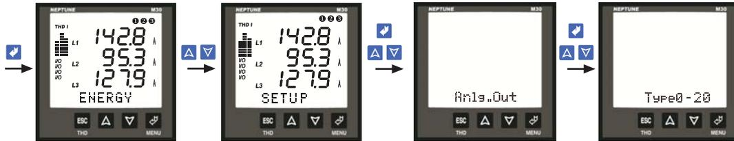
In device, this feature gives the possibility that observing the measured values by other devices with converting these values in to 0-20 mA or 4-20 mA current data. The below parameters can be set as analog output in device.
