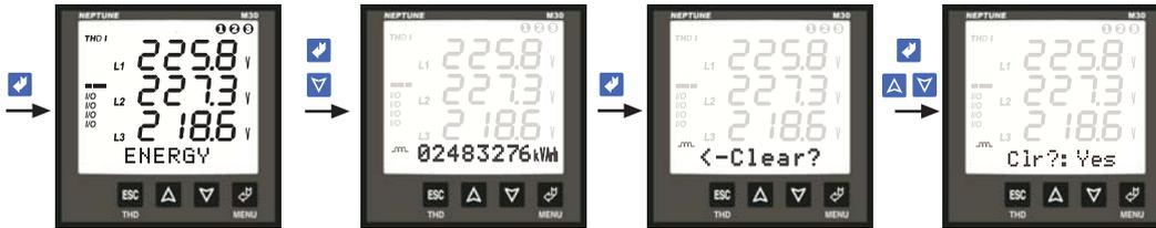
Figure 41: Clearing the Inductive Reactive Energy value
