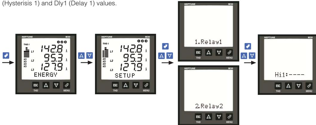
**Figure 26:** Setting the high (over) value for the 1st parameter
