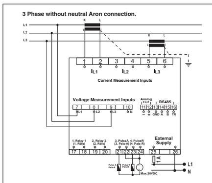
Figure 8: ARON connection (3 phase without neutral connection)
