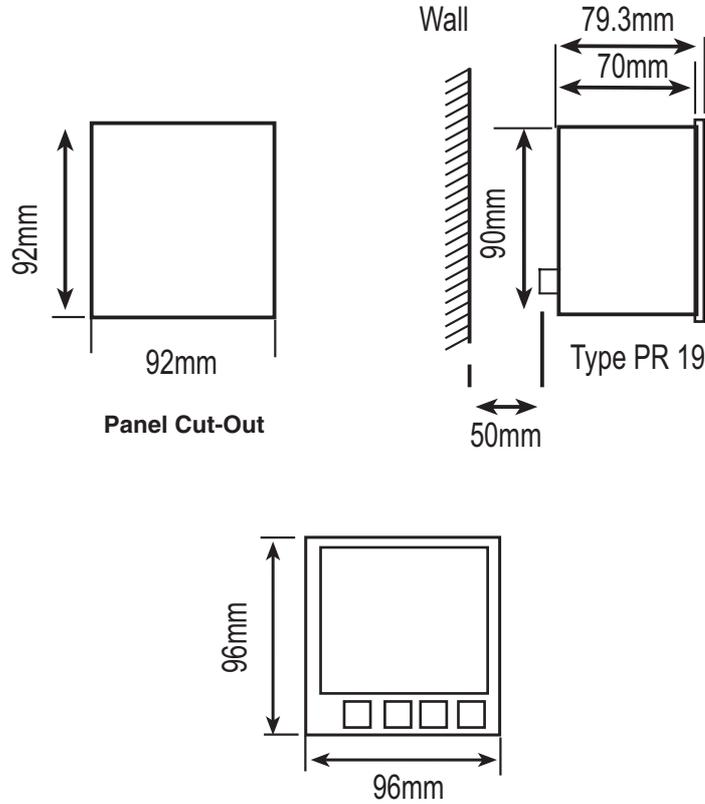
**Figure 5:** Dimension and the panel cut-out.
