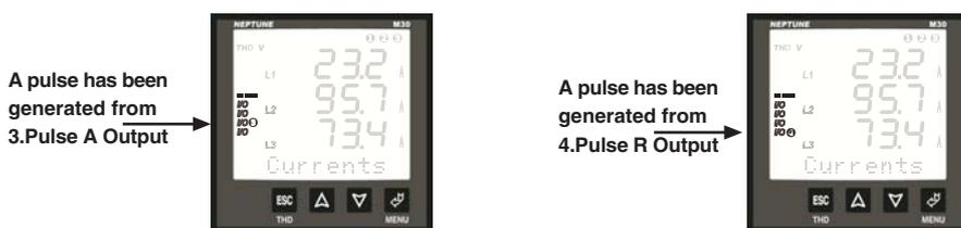
Each time the consumed energy increases by an increment of "Prm", a pulse, as long as the "Dur" value entered (msec), is produced in the Pulse Outputs.
