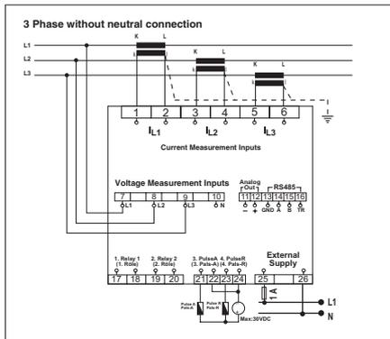
Figure 7: 3 phase without neutral connection
