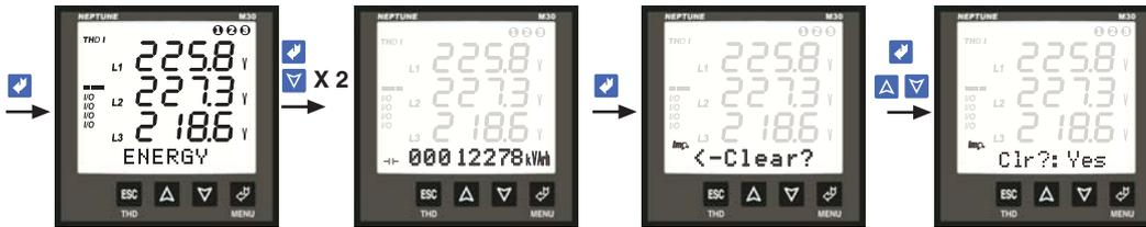
Figure 43: Clearing the Capacitive Reactive Energy value
