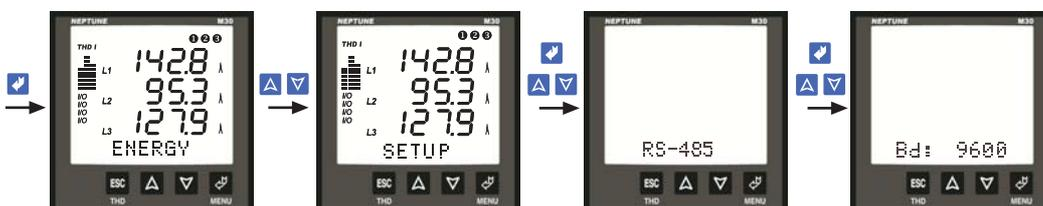
Figure 18: Setting the baud rate value
