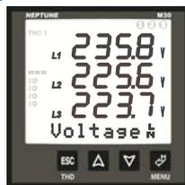
**Voltage<sub>t</sub>** Measured phase-phase voltage value VL1-2, VL2-3, VL3-1
