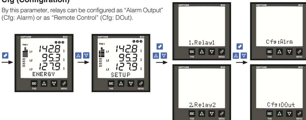
Figure 24: Relay control type setting
