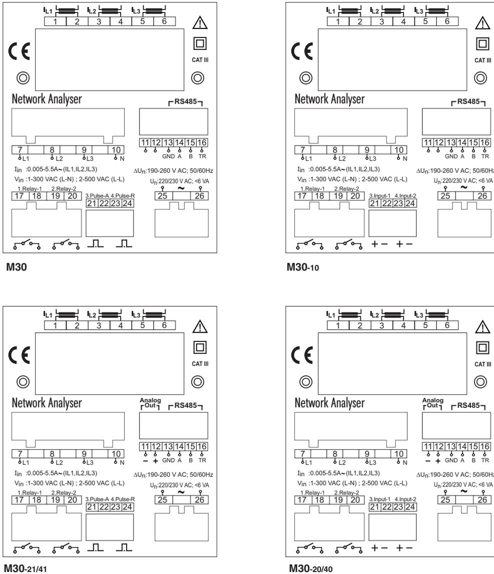
Figure 4: The terminals on the rear panel.
