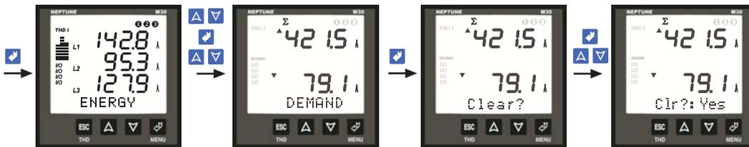
Figure 63: Clearing the Min. / Max.  $\Sigma$  I
