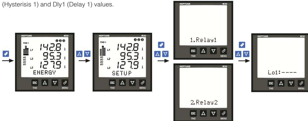
**Figure 27:** Setting the low (under) value for the 1st parameter
