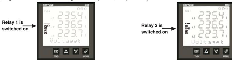
Figure 23: Active relays are displayed on LCD.
