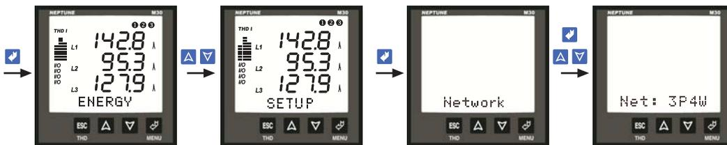
Figure 13: Setting the type of system connection
