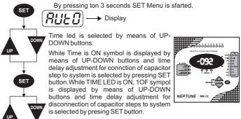
A value between 2-1800 sec. Is adjusted by using UP-DOWN buttons.
