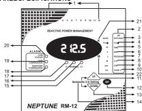
On the front panel of RM Series, there are warning LEDs display and 3 buttons for Setting
